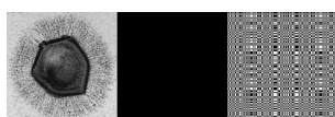
Fig. 1. Specimen (the mimivirus [5]) and reference object (the uniformly redundant array [6]) used in simulation. Both specimen and reference objects are of size 256 \times 256 pixels, and are separated by a 256 \times 256 zero-valued region.
