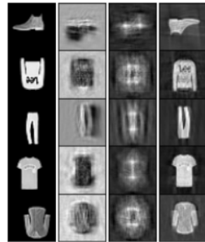
Figure 4: Comparison with ALM. 1 st column contains groundtruth images, 2 nd , 3 rd and 4 th column are reconstructions from ALM, U-Net-B and U-Net-A respectively.
